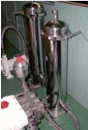
SUPPLY TO D440 and D660: Stainless steel double pre-filter, bronze low pressure pump, carbon membrane tubes.
